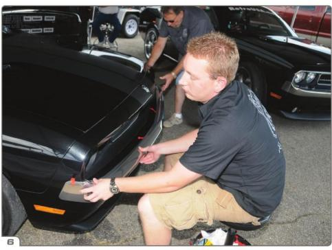
Gary Green holds one end while Daryl makes certain the bumper is properly aligned. Time is taken to be sure that the bumper is exactly right; Daryl worked from the center of the car to the ends, making sure the bumper has not shifted. By exposing a small amount of adhesive at each end point, the bumper is securely held to the car while Daryl prepares to strip out the ribbons.
